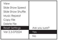
Press ▼ buttons to select the Reset Settings mode. Yes: Reset the Original setting No: Default Setting
