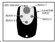
**To transmit channel 9, 10, 11 or 12:** Press the LevelShift button twice. This shifts the buttons to level 3 (channels 9–12). Then press the corresponding button within the next 7 seconds. For instance, to transmit channel 10, press the LevelShift button twice, then press button 2. The LED on the remote control flashes three times, pauses, flashes three times, etc.: this indicates **level 3.**
