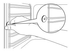
2. Pull the rear shelf support rail away from the side wall and remove it.
