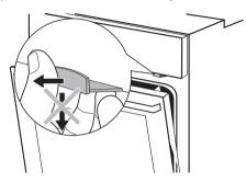
Activating the door lock: Pull the door lock forward until it locks in place. Deactivating the door lock: Push the door lock back into the panel.
