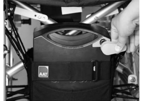
Plug the power cable's plug into the socket on the movilino.
