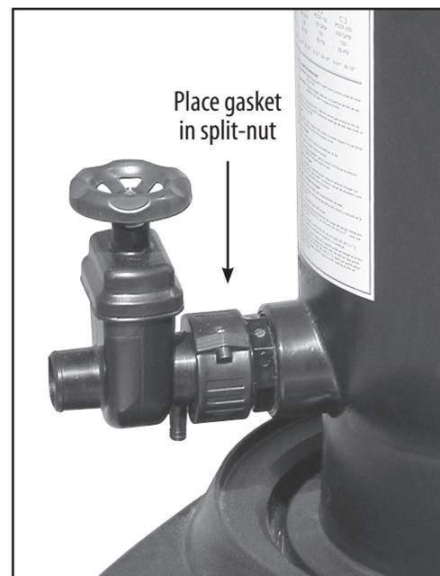
6. Place the other 1 1/2" gasket in gate valve split-nut and thread onto 2" x 1 1/2" MPT union fitting.
