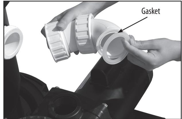
4. Make sure gasket is in place on elbow assembly and install onto tailpiece. Elbow side has label "inlet." Place gasket in pump end of elbow assembly and attach to discharge on pump. Insert snap pins through motor base and into filter base.
