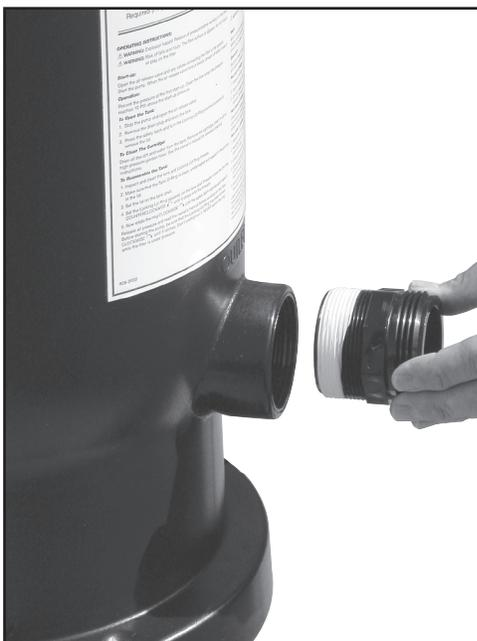
5. Wrap 3 or 4 turns of Teflon tape (provided) on 2" x 1 1/2" MPT union fitting and install into "outlet" of filter.
