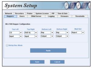
Each of the bottom two hoppers can be selected as an Output or a Reject. Input
