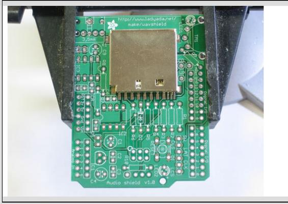
We're going to the SD card first. While surface mount parts are a little tougher than thru-hole, this piece has pin spacing of 0.1" so it is quite easy. Doing it first also gives us lots of working room. The holder should 'snap' perfectly into place thanks to two bumps on the bottom.
