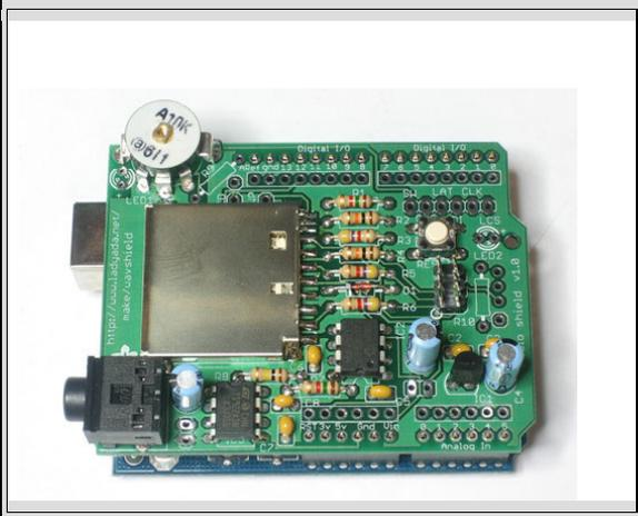
Place the shield PCB onto the Arduino so that all the holes match up with the header.
