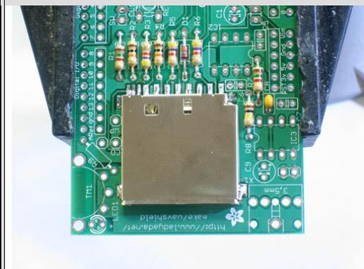
Place the capacitor right next to R7. Ceramic capacitors are non-polarized and can go in 'either way'
