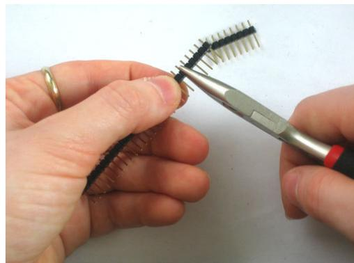
Next, break the 36-pin header strip into smaller sections so that the shield can be placed on the Arduino. You can use pliers or diagonal cutters. Clip off 2-6pin and 2-8pin pieces.
