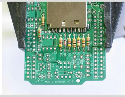
Finish up the resistors by placing R8 (100Kohm), R1 (1.0K) and R7 (1.5K). In the photo, R1 is shown as 1.5K...this is a mistake! (It was too flakey for me and I reduced the resistance). Make sure you place a 1.0K resistor in R1! Solder the components
