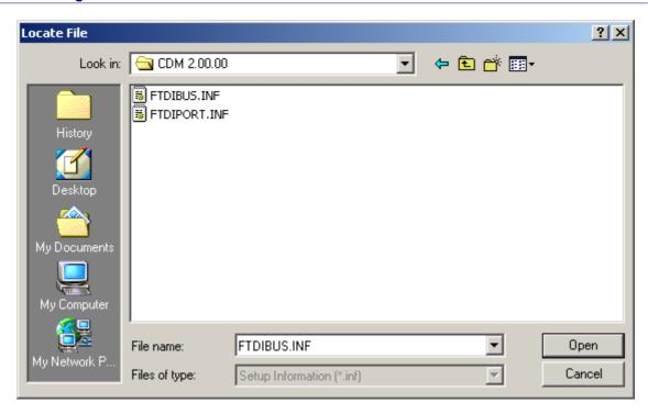
Locate the folder containing the latest drivers downloaded from the <u>FTDI web site</u> above and click "Open", then click "OK". The PC autoselects the correct INF file, in this case FTDIBUS.INF. Once Windows has found the required driver .INF file, click "Next" to proceed.
