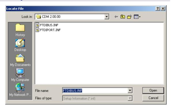
• Locate the folder containing the latest drivers downloaded from the <a href="FTDI">FTDI</a> web site</a> above and click "Open", then click "OK". The PC autoselects the correct INF file, in this case FTDIPORT.INF. Once Windows has found the required driver .INF file, click "Next" to proceed.
