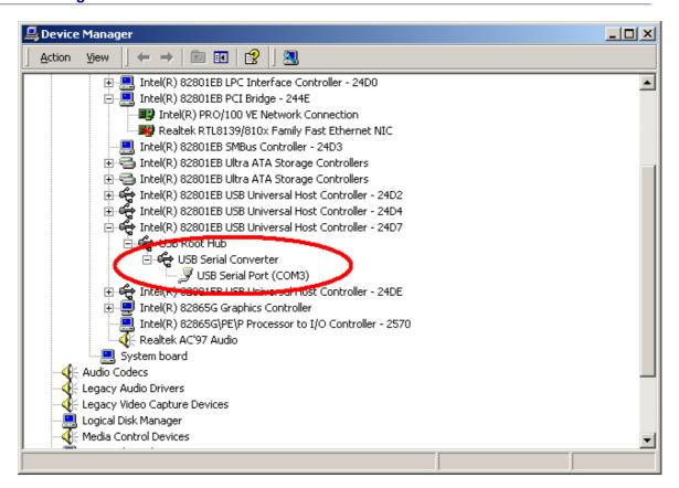
• In the case of the FT2232, port A of the FT2232 will be installed as COMX and port B will be installed as COMX+1 where COMX is the first available COM port number.
