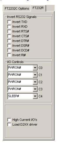
Like the FT2232C, the FT232R supports High Current IOs. Setting this option will enable the high output drive level. The UART IO pins will drive out at 12mA instead of their normal 4mA.
