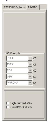
Like the FT2232C, the FT232R supports High Current IOs. Setting this option will enable the high output drive level. The FIFO IO pins will drive out at 12mA instead of their normal 4mA.
