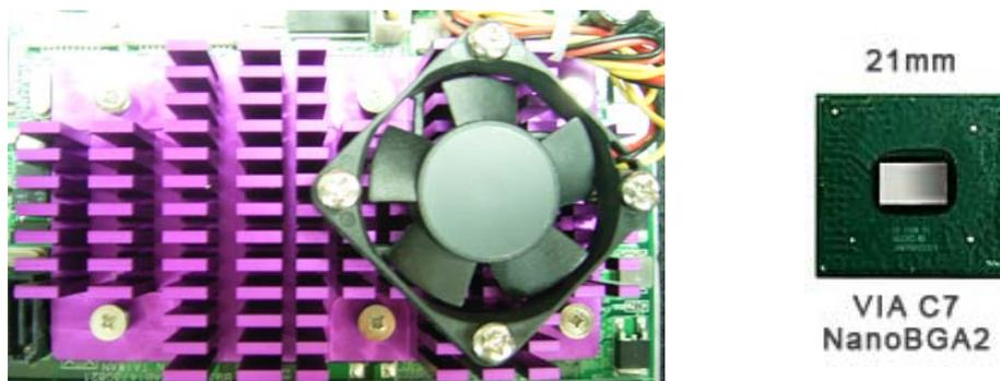
When user is going to exercise WADE-6010, you must check the power connector of cooler module of CPU, and then follow the position to connect the power line, see the below image of demonstration.
