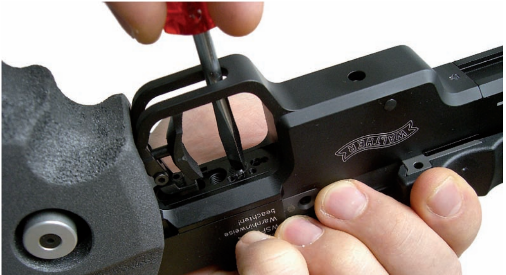
Adjusting the sear point (or sear point travel / pawl intersection)
