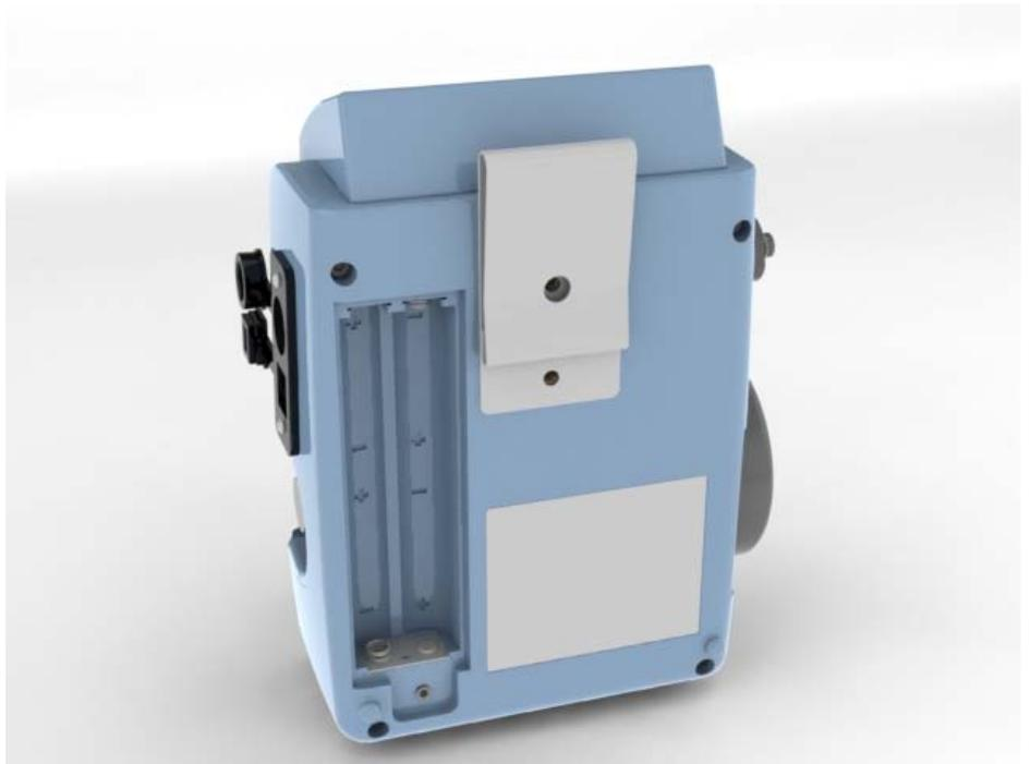
**Figure 2–5.** Bottom Battery Door and Belt Clip
