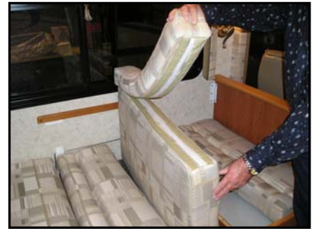
Figure 5-5. Filler Strip Attached to the Seat Portion
