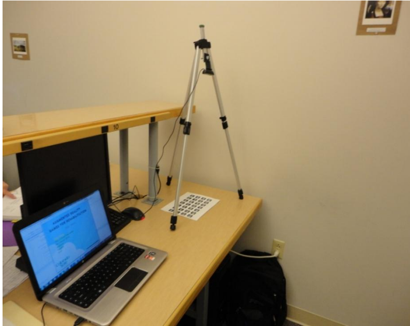
Figure 3. AR Games Hardware System : Tripod with a webcam, AR marker and a laptop.
