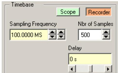
In Transient recorder mode, shown to the left, the user selects the sampling rate and the number of samples. This is closer to the kind of setup used in the analyzer mode.
