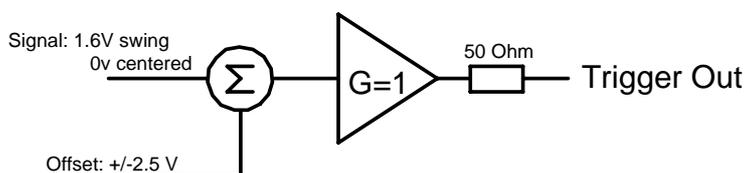
The output swing is 1.6 V ( $\pm 0.8$  V) when unloaded and 0.8 V when terminated on 50  $\Omega$ . The rise and fall times are 2.5 ns typical. The offset can be adjusted, by software control in the range [-2.5 V, +2.5 V] unloaded, or [-1.25 V, +1.25 V] into 50  $\Omega$ . The maximum output current capability is  $\pm 15$  mA. As the output is retro-terminated, it is possible to drive a 50  $\Omega$  line unterminated (HiZ) without loss of performance.
