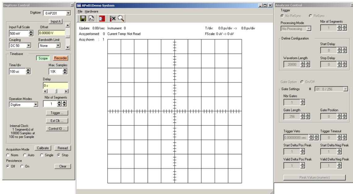
APx01Demo displays three independent windows, a Digitizer Control window, an Analyzer Control window, and a display window. The Control windows contain functions that allow you to manipulate the acquisition parameters of the card. In order to display an acquired waveform, connect a signal to the input, and then select the Auto acquisition mode at the bottom of the Control panel. A waveform should appear in the display. Note that this is best done with the Operation Mode: Digitizer.
