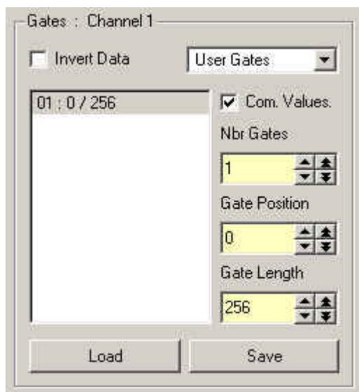
For the User Gate mode shown below the number of gates together with their length and starting position can be modified as needed. As soon as more than one Gate is available the field to the right of the # sign can be used to select a gate for editing. Note that the Gate Length is to the left of the Gate Position, which implies that it has priority. This means that Gate Position will be forced to satisfy the relation
