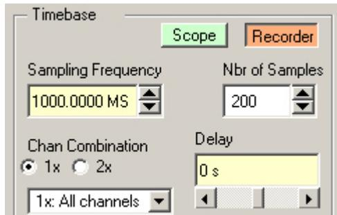
In Transient recorder mode, shown to the left, the user selects the sampling rate and the number of samples. This is closer to the kind of setup used in the analyzer mode.
