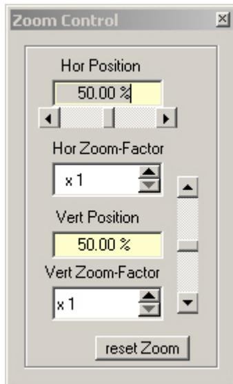
This will activate the Zoom Control menu shown here. The horizontal zoom is controlled by the Hor Position, with 50% in the middle of the screen. The vertical zoom is controlled by the Vert Position, with 0% in the middle of the screen and +50% meaning that the display should be shifted up by  $\frac{1}{2}$  the screen height. New zoom values can be used on existing data by pushing the Reread button in the Digitizer Control window.
