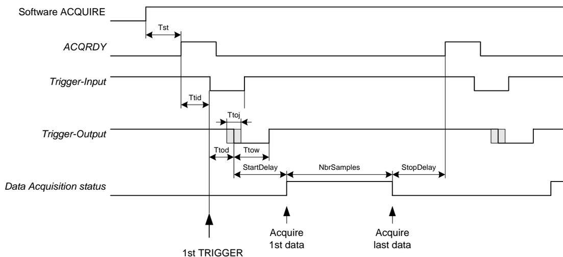
the individual trigger time stamps makes it possible to determine the time from one trigger to any other trigger in the sequential acquisition. The TTI resolution sets the resolution of the trigger time stamps.
