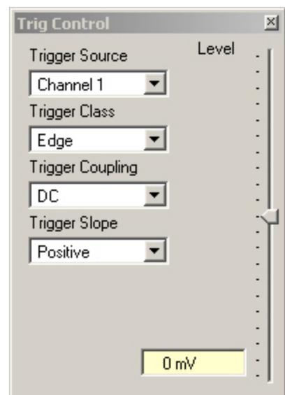
The *Coupling* setting can be AC, DC, or Hfrej coupling. Use the *Level* section to set the desired trigger level. The External Trigger Source menu will also allow selection of the desired Trigger Range and Bandwidth. The relationship between coupling, trigger source, and trigger level was discussed in section 3.3.3, **Trigger Level**.
