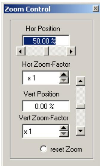
This will activate the Zoom Control menu shown here. The horizontal zoom is controlled by the Hor Position, with 50% in the middle of the screen. The vertical zoom is controlled by the Vert Position, with 0% in the middle of the screen and +50% meaning that the display should be shifted up by 1/2 the screen height. New zoom values can be used on existing data by pushing the Reread button in the Digitizer Control window.
