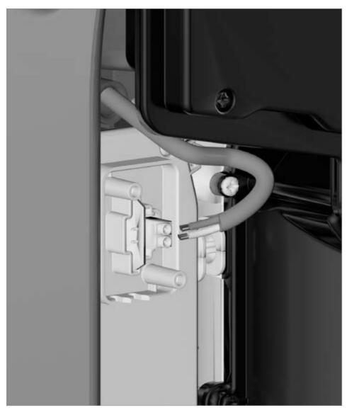
Once the cable has been passed through the hole, connect each end to its respective terminal, placing each one in the right path and then close the box.
