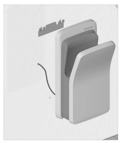
Place the ffuuss™ hand dryer on the wall mooring, remove the air intake filter and fix the unit via the inner hole. Insert the filter and connect the unit.
