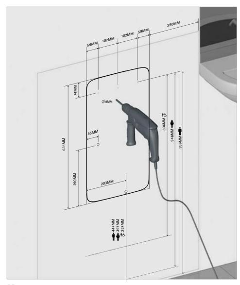
Place the hand dryer ffuuss™ template against the wall where it will be installed and make the holes according to the diagram. Check beforehand if there is a direct cable to the electricity network or if the hand dryer has to be connected using a plug.
