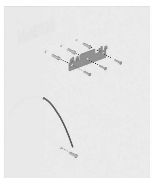
Once the marks have been made, attach the mooring to the wall and prepare the cable to the electricity network.
