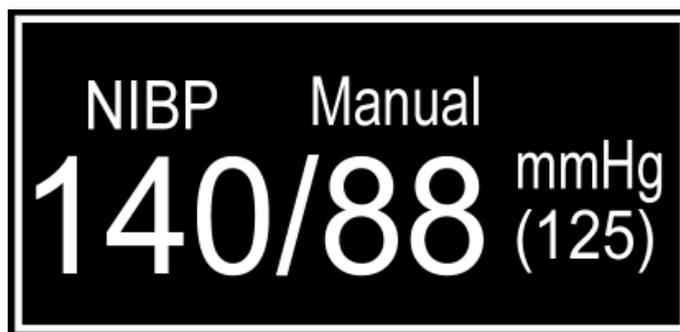
This section displays the operating mode for NIBP (Automatic, Manual or STAT) and the numeric information for the last NIBP reading taken. The information supplied is in the format Systolic/Diastolic and (MAP) mmHg values or Systolic/Diastolic mmHg and Pulse Rate ♡. The selection between (MAP) or Pulse Rate ♡ can be made in the NIBP Options menu.
