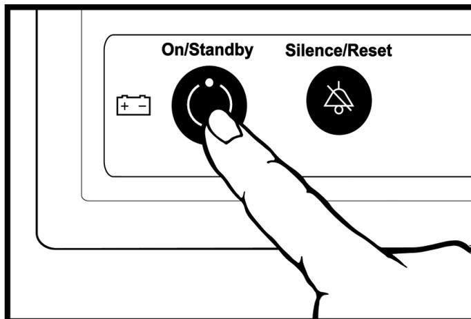
Each time the monitor is turned “ON”, a brief electronic song will play while the Power On Self-Test (POST) is conducted to ensure that its internal circuits are functioning properly.
