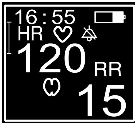
This section contains the current monitor time and Battery Charge Status icon.
