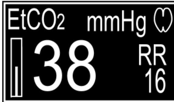
In the model 9405, this section displays the numeric values for both EtCO<sub>2</sub> and Respiration Rate and a flashing visual icon for the Respiration Rate.
