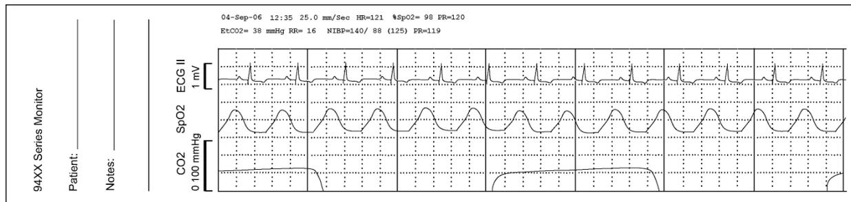
To print waveforms, press and hold for two (2) seconds the FREEZE, PRINT, MAIN pushbutton (L) while in the Main display screen. The waveforms being displayed will print based on the Print Traces selections in the Parameters menu. Refer to Page 96, PARAMETERS MENU for the Print Traces selections.
