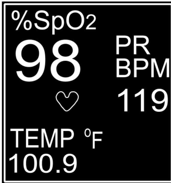
In the models 9403 and 9405, this section displays the numeric values for %SpO<sub>2</sub> and Pulse Rate and a flashing visual icon for the Pulse Rate. In the model 9404, this section displays the numeric information and a flashing visual icon for the Respiration Rate.
