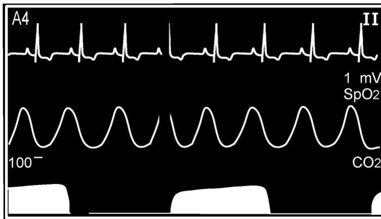
During normal operation, this section (Refer to Figure 14 on the previous page) displays the traces that have been selected in the Parameters menu. Up to three (3) traces can be selected. The traces are displayed in an erase bar format.
