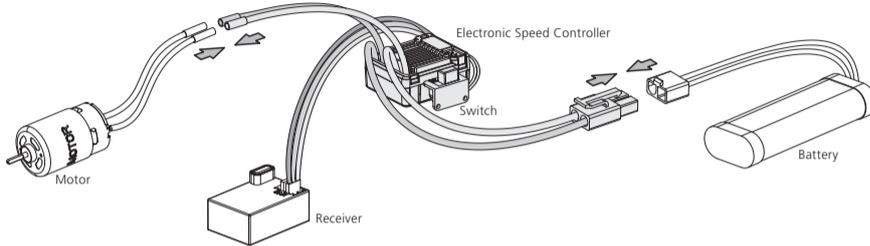
Turn off the ESC switch, wire the battery, motor, ESC, servo, receiver according to the following diagram. Check the wiring to ensure all connections are correct before getting into the next step.
