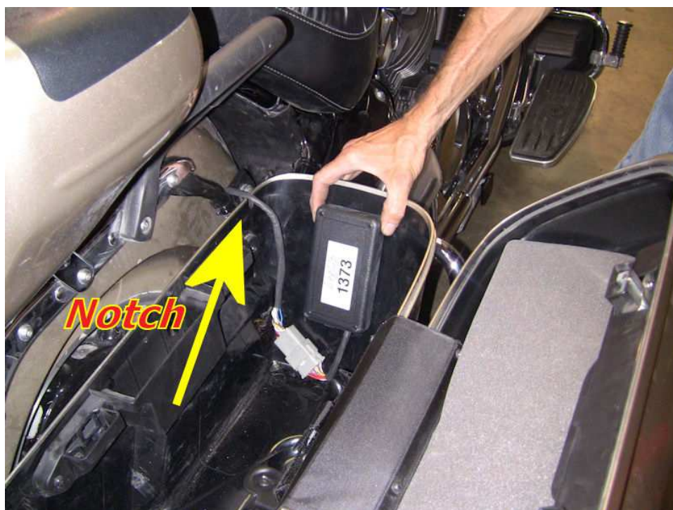
Attach Velcro inside Saddlebag for the Computer Mount Computer as shown.
