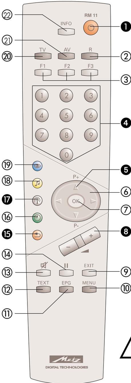
The remote control sends commands to the TV set by means of an infrared signal. You must point it towards the TV set when using it. Note that the remote control may interfere with the operation of other devices which use infrared signals (such as infrared headphones).
