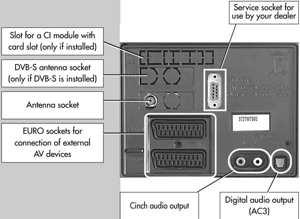
***👉 The digital audio signal (AC3) provided by the set can be connected to external devices with the aid of an optical audio cable ("Tos-link", available as an accessory).***
