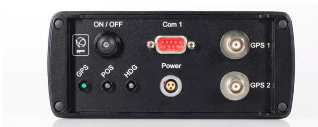
**ON/OFF:** To turn on the 4011 GPS Compass press the Power button. The power LED lights up in red.
