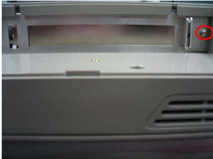
**Step 7.** Close back cover to the chassis, and fasten securely with all screws.
