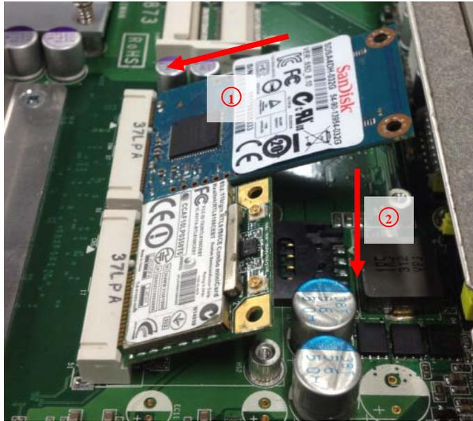
**Step 6.** Use screws to fasten the Mini Card.
