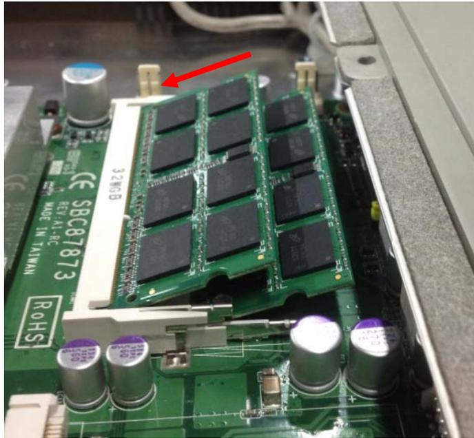
**Step 6-2.** Install the memory module into the socket and push it firmly down until it is fully seated. The socket latches are levered upwards and clipped onto the edges of the SO-DIMM.
