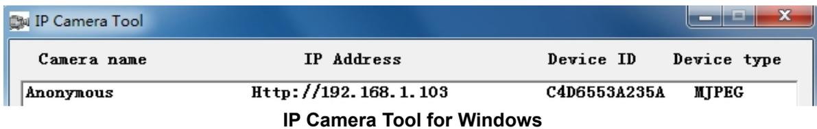
The IP camera tool should find your camera's IP address automatically (your IP address may be different) after you plug in the network cable. If not, please make sure that DHCP is enabled on your router and that MAC address filtering, firewalls and anti-virus are disabled temporarily until the camera is set up.
