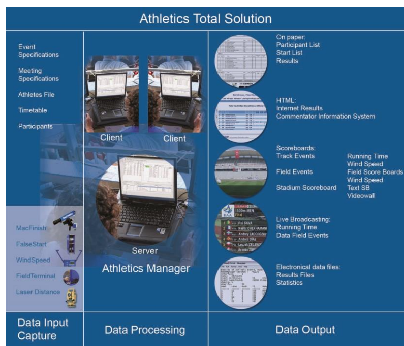
Figure: Data is being entered in input equipment (left), then processed by AthleticsManager (center) and next exported to output equipment (right).
