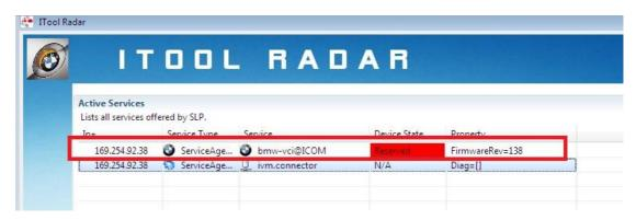
$\hbox{@Open EasyConnect, Set as follows}, \ \ \hbox{The} \quad \hbox{IP address} \quad \hbox{must be Correct}$
