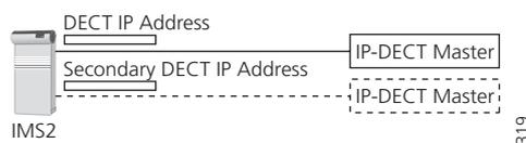
Figure 31. Redundancy achieved by connecting IMS2 to two IP-DECT base stations and setting primary and secondary IP addresses.
