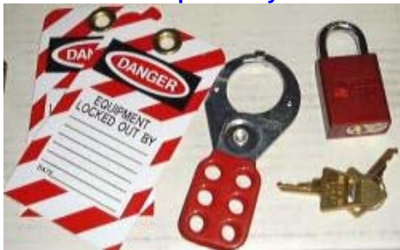
Example of lockout tags, lockout hasp and keyed lock
