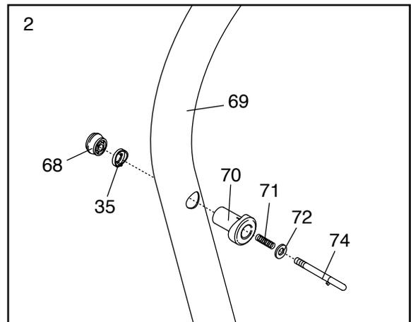
3. With the help of a second person, carefully tip the Uprights (69) down as shown. **Make sure that the Extension Legs (102) remain in the Uprights.**
