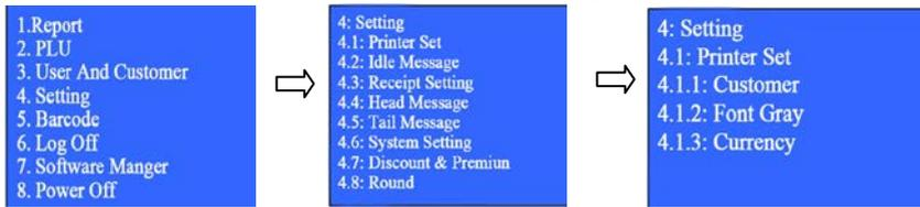
2) Input the printing font gray level that according to your demand.( Printing font gray level from 1 to 10. The printed words are more black if the font gray level higher, but the printer mechanism will easy to wear)
