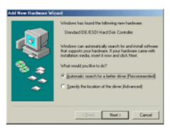
Windows will install its resident driver – 'Standard IDE/ESDI Hard Disk Controller' for the external CD-RW. After the necessary files are copied into your internal hard disk, a screen will appear as the figure, click *Finish*.
