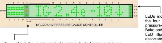
The units of the pressure display are indicated by one of three LEDs in the display area. The centre orange LED indicates that mBar has been selected, the green LED above it indicates Pascal and the green LED below indicates Torr.
