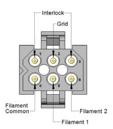
Base connections of AIG1x gauges.
