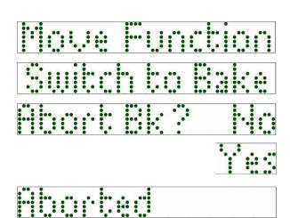
Start Bake by turning the Function Switch to BAKE and press ENT.
