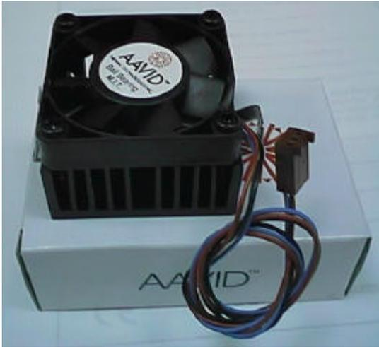
Figure 3: Boxed Celeron™ Socket370 Processor & Heat sink support
