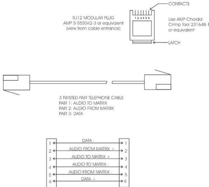
FIGURE 16. RJ12 Intercom Cable Wiring
