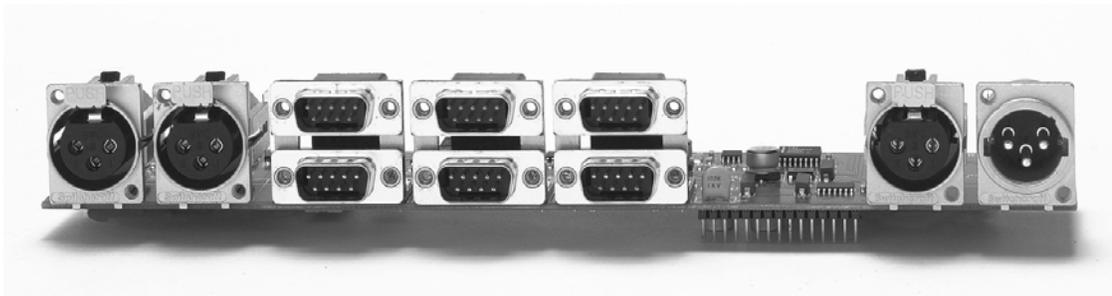
**FIGURE 12.** KP 832 Connector Option Board
