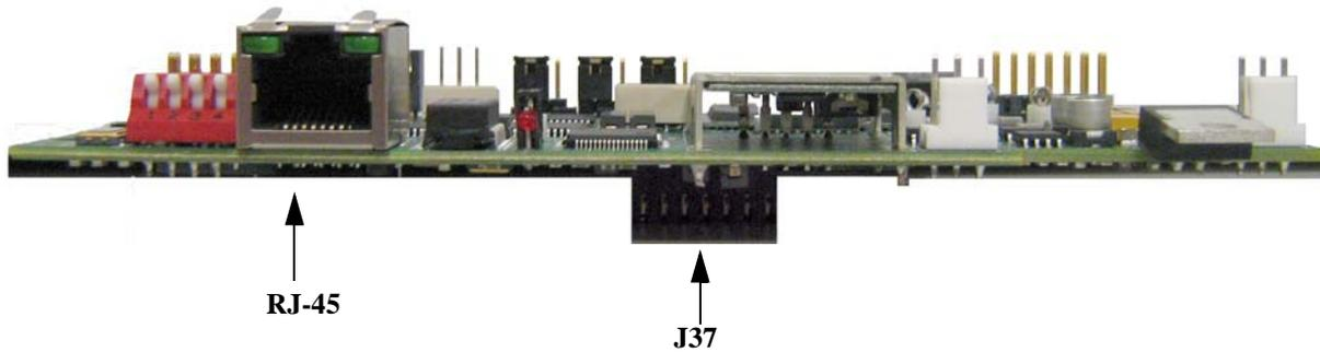
3. Connect the **RJ-45 extension connector cable** to the RVON-1 board.
