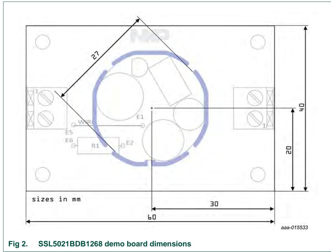
**Fig 2. SSL5021BDB1268 demo board dimensions**
