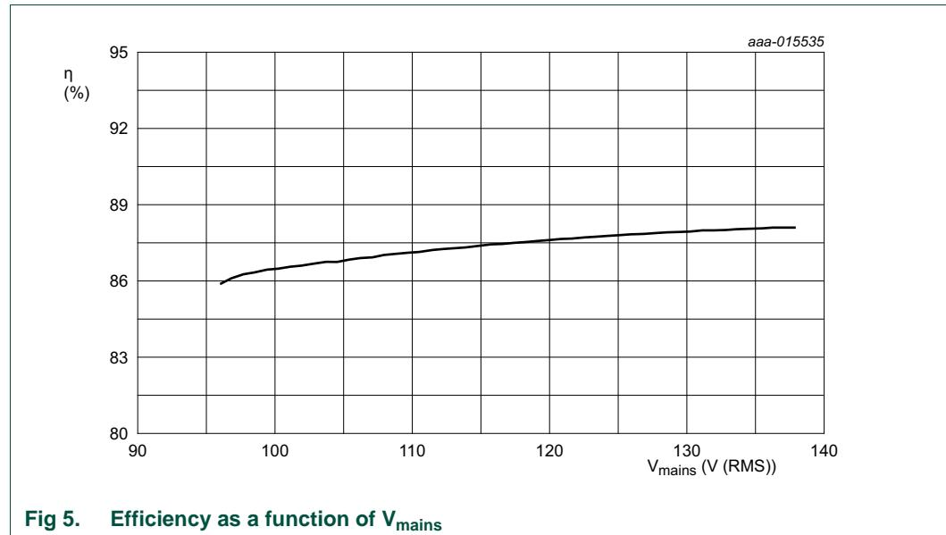
Fig 5. Efficiency as a function of  $V_{\text{mains}}$
