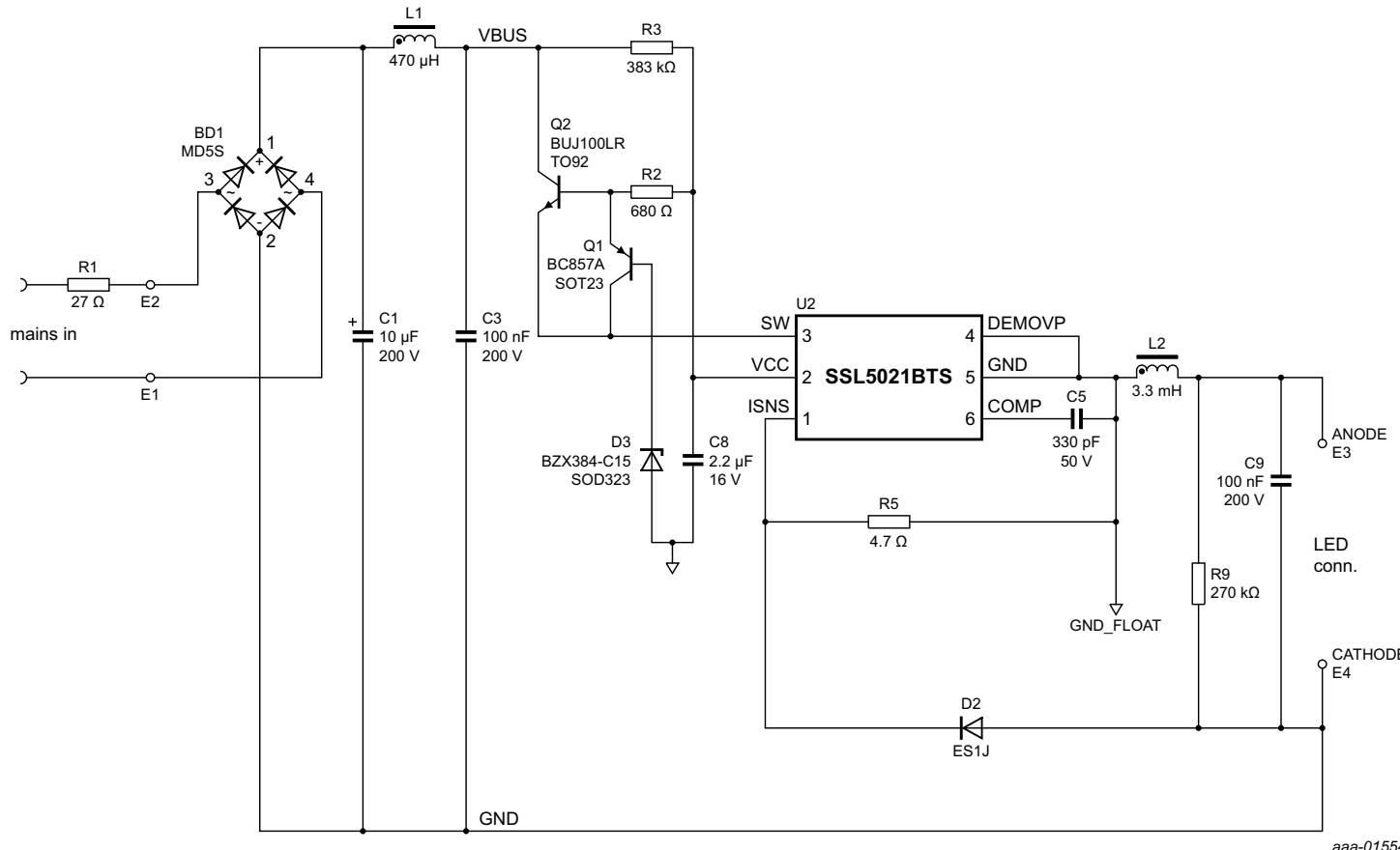
Fig 11. SSL5021BDB1268 demo board schematic diagram
