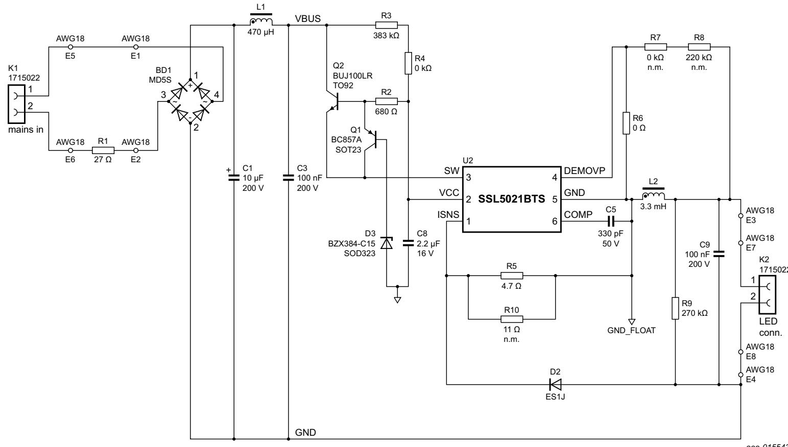
Fig 12. SSL5021BDB1268 demo board schematic
