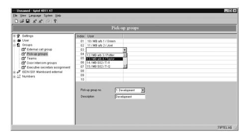
Pick-up and pick-up from the device connection is only permitted for telephones entered in the pick-up group.
