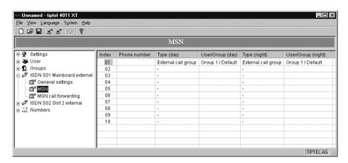
The destination type can be set via a Combo-Box. If *External call group* is set, a list of the external call groups is displayed in the adjacent column (in this case *Day*):
