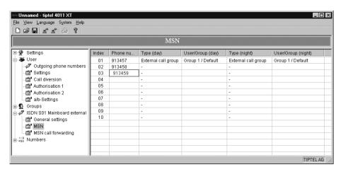
The *Port* column provides a list of the external ISDN connections. In the example, only the So1 on the mainboard is switched to external.
