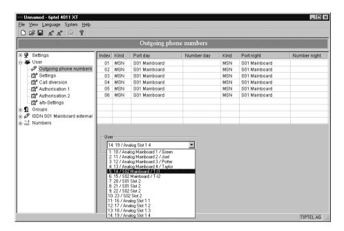
When restarting the System, no assignments are entered as no MSNs have been defined either.
