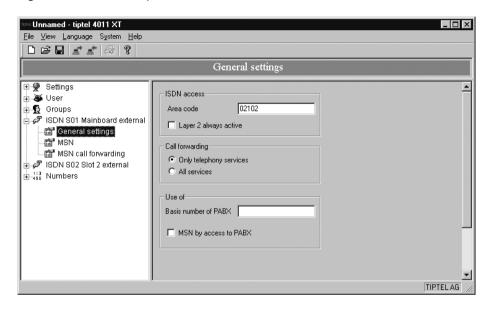
Under *Use of*, the MSN and DDI options can be activated simultaneously. This is not an advantage in Germany as only DDIs exist for a point-to-point connection. In contrast, MSNs and DDIs can be defined in France, for example.
