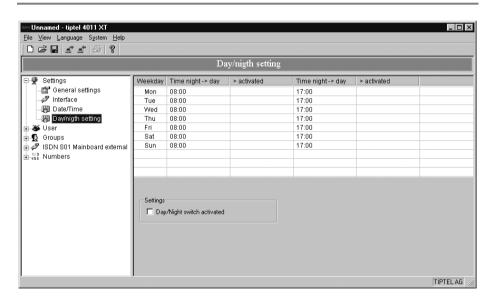
The Telephone System can be switched manually or automatically from day to night activation and vice versa. The same parameters are used in both cases.
