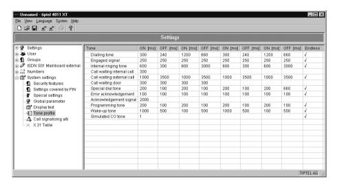
The ringing and control tones are normally in the form of endless loops with 4-level tone sequences. One level comprises switching tone ON and tone OFF. The tone frequency is 440Hz.
