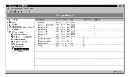
Each call source can be assigned a variable signal sequence and the number of repeats.
