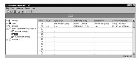
The index is not identical to the DDI or the internal call number. In the example, DDI 40 has been assigned to subscriber 12 for day and night.
