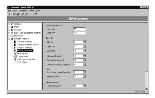
Compiled here are numerous parameters for the Telephone System as a whole. Importance for configuration is the setting of the call number of the virtual extension that must be called by the PC program (for connection setup via ISDN).
