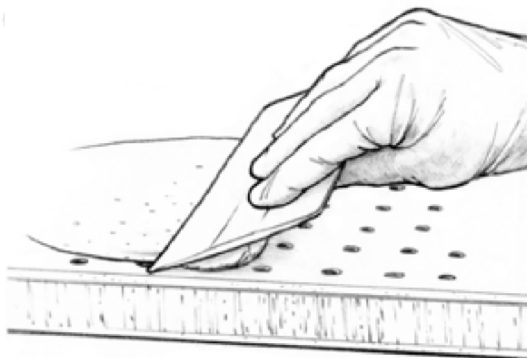
Figure 3. Fill any remaining voids and holes and fair the surface with an epoxy/407 mix.
