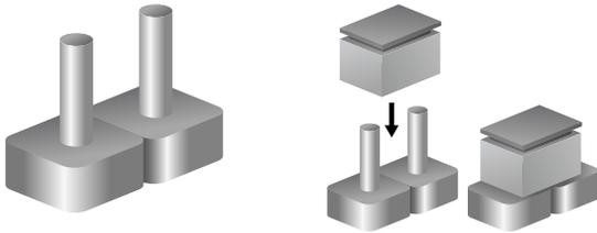
Three-Pin Jumpers: Pins 1 and 2 Are Short
