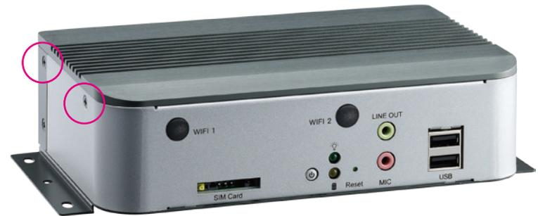
2. Lift the cover upward then remove it from the chassis.
