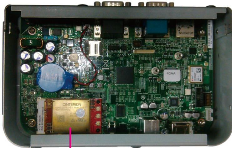
Mini PCI-E slot for WWAN module installation
