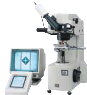
HM-113 Reduce individual differences in visual measurement with the TV monitor. The statistical calculation function reduces operation time.
