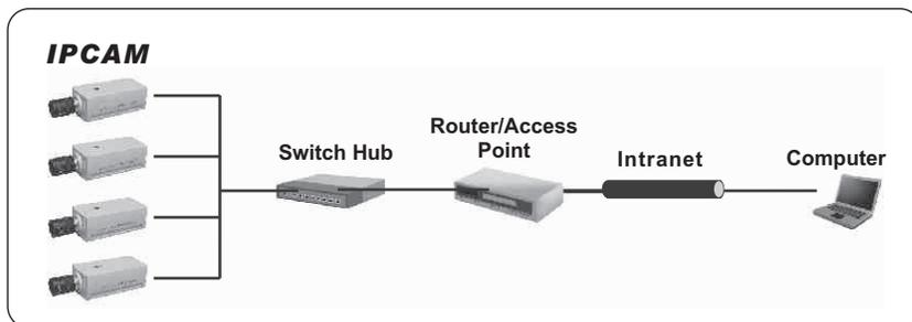
1. Cat 5 cable must be used in condition of connection via router, DSL modem and hub.
