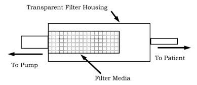
To ensure there is no entry of fluid into the pump the Hydrophobic Shut Off Valve Filter MUST be fitted as shown above.
