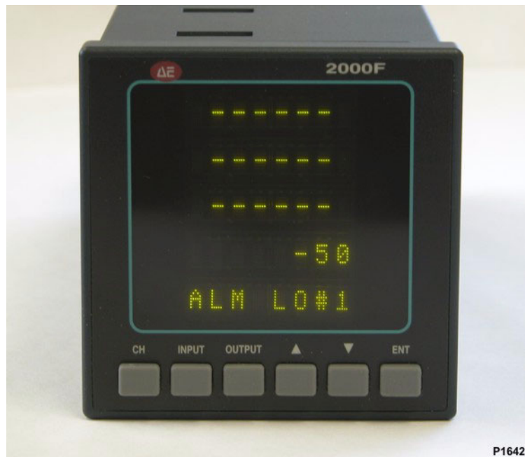
Figure 4-14. Example ALARM reading
