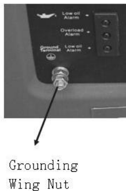
Figure 15- Grounding nut location
