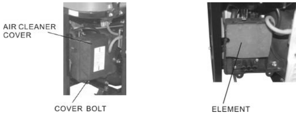
Figure 30- Removing the air cleaner casing.
