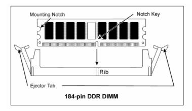
To remove the DIMM modules, push the two ejector tabs on the slot outward simultaneously, and then pull out the DIMM module.
