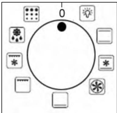
The oven function selector knob should be used to select the particular mode of cooking that you require. The appliance will utilise different elements within the oven cavity, depending on the oven function that you select. When a function is selected, the power indicator light will come on.
