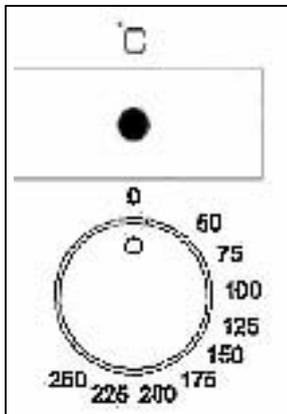
The oven thermostat control knob sets the required temperature of the oven. It is possible to regulate the temperature within a range of 50 - 250°C.
