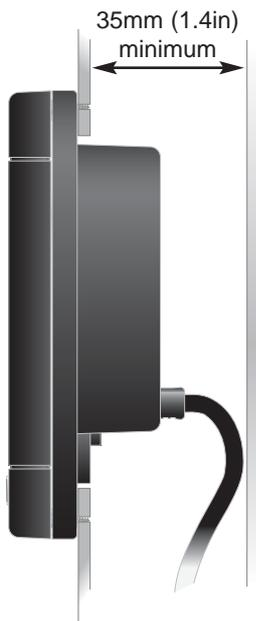
Fig 4.2 - Clearance Required Behind Bulkhead
