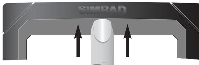
*Fig 4.4 - Removing Bezel*
