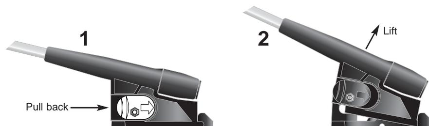
Fig 4.13 - Removing Masthead Transducer
