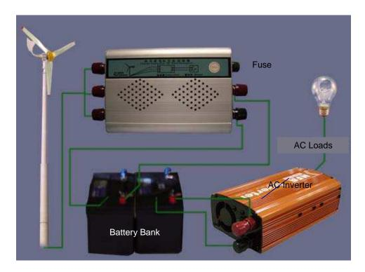
The general electrical configuration or setup is illustrated in Section 2 and above. The tower should also be grounded for electrical safety. In most cases the loads will probably be 240VAC/50Hz and will obtain power via an AC inverter connected to the battery bank.
