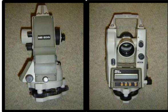
Figure 37. The Nikon NE-20S Digital Theodolite
