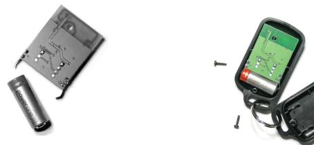
Replace the screws and screw the unit together.
