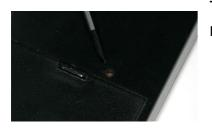
The learn button is in a small hole on the back of the receiver, just above the battery compartment.
