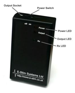
The receiver has two simple controls and 3 LED's.
