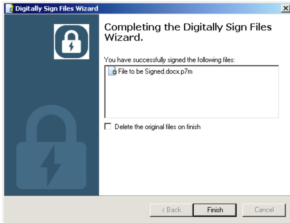
8. The output of the Digitally Signed file will be in a new format (.p7m)
