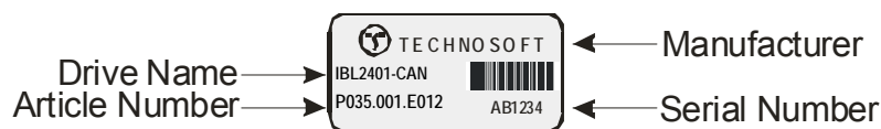
Figure 3.5. IBL2401-CAN (CANopen execution for Brushless and DC motors with incremental encoder) Identification Label
