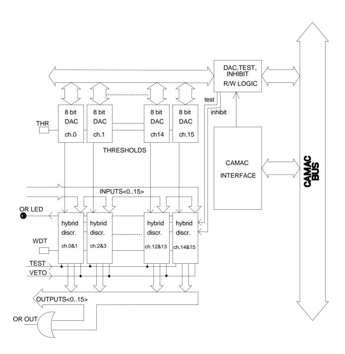
Fig. 1.1: C207 Block Diagram
