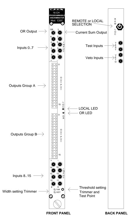
Fig. 2.1: C207 Front and Back Panels
